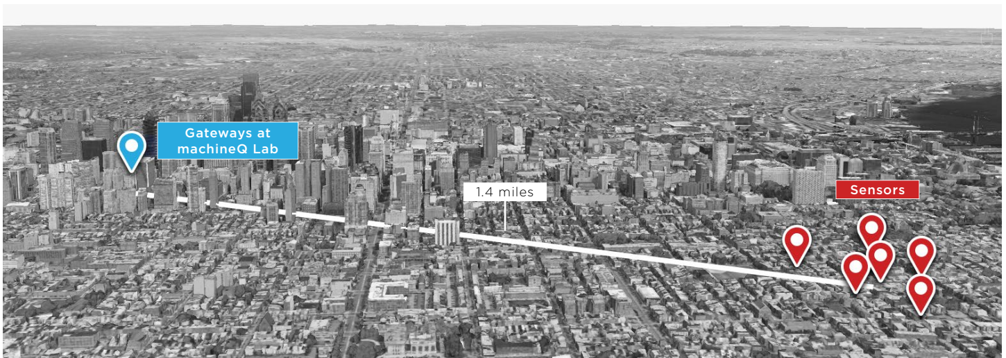
Figure 5. Shows distance between sensors and a gateway in the office that received packets
