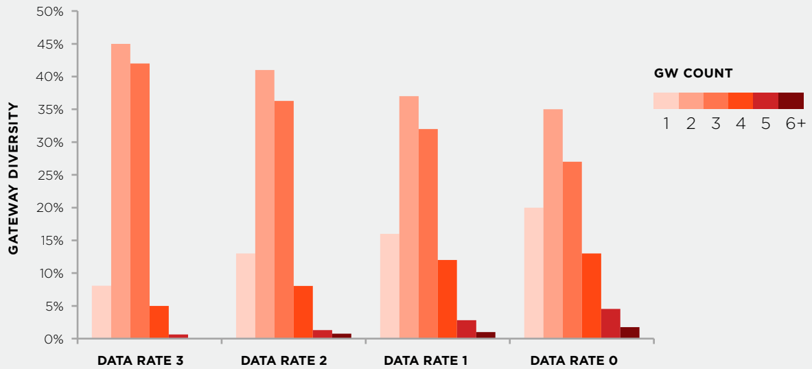
Figure 9. Gateway diversity recorded throughout the study. Gateway diversity is defined as the % of packets received by multiple gateways.
